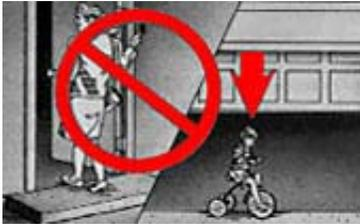
When using the push-button or transmitter, keep the door in sight until it completely stops moving.
